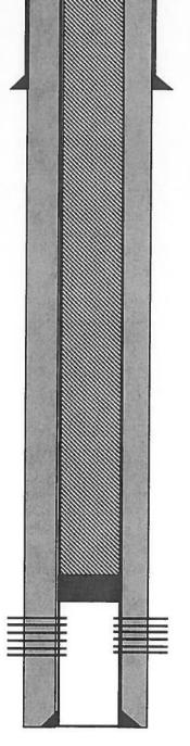
5 ½" 14# Casing Set @ 40'. Cemented w/ 5 sks. Hole size 7-7/8"
