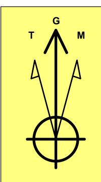
**Azimuths to Grid North** True North: -0.35° Magnetic North: 6.40°
