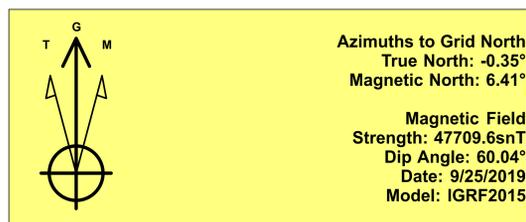
To convert a Magnetic Direction to a Grid Direction, Add 6.41°
