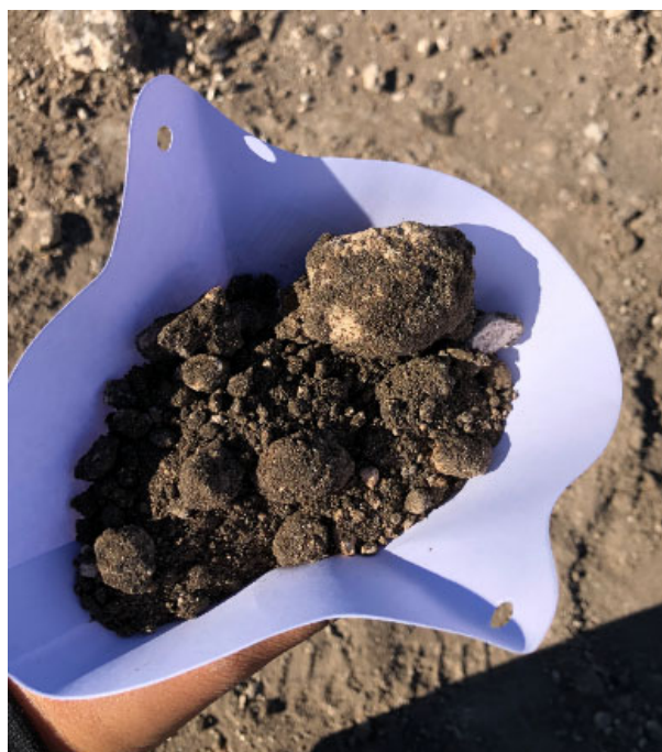
Figure 3 - Paint Filter Test (11/18/19)
