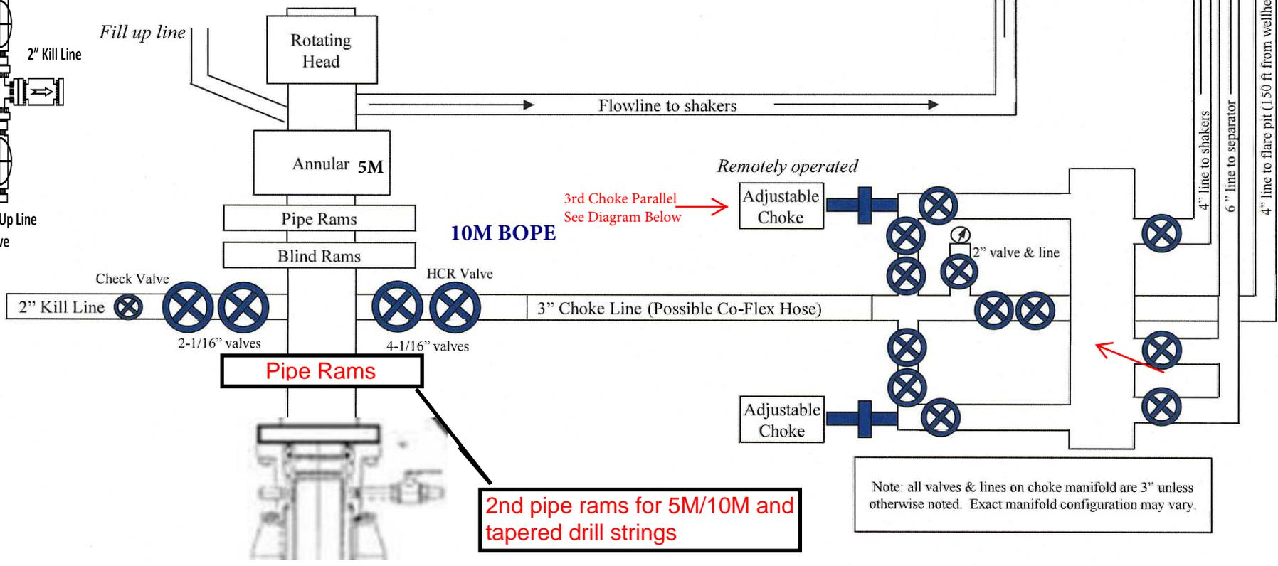
2nd pipe rams for 5M/10M and tapered drill strings
