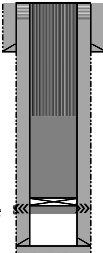
4-19-2021: Tag TOC inside casing at surface. Cut off WH, TOC in annulus was 16'. Install P&A marker. Mix and pump 24 sx class G to top off cellar
