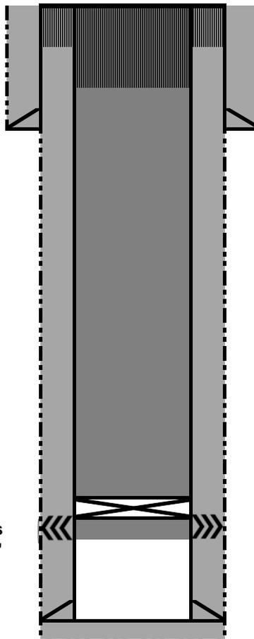
11-24-2020: Tag fallback at 100' in 4 1/2" casing, 30' in 7" x 4 1/2" annulus. Mix and place 30 sx top off plug with polypipe to surface
