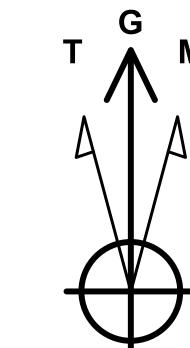
Azimuths to Grid North True North: -0.46° Magnetic North: 6.03°
