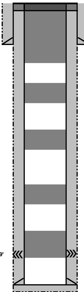
1-18-2021: Plug 6: Top off with 34 sx Class G cement. Install P&A marker.
