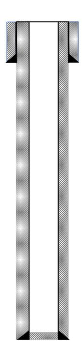
8-5/8", 24# J-55 Casing set @ 132.5' RKB Cemented w/ 200 sks Class B cement w/ 2% Calcium and ¼#/sk CF Circulated 6 bbl cement to surface
