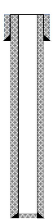
8-5/8", 24# J-55 Casing set @ 120' RKB Cemented w/ 100 sks Class B cement w/ 2% Calcium and ¼#/sk CF Circulated 8 bbl cement to surface
