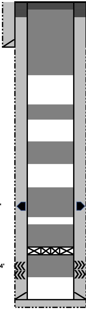
11-03-2021: Cut off WH, TOC in 8 5/8" x 5 1/2" annulus 100', in 5 1/2" casing 23'. Top off with 42 sx cement. **RELEASED RIG.**
