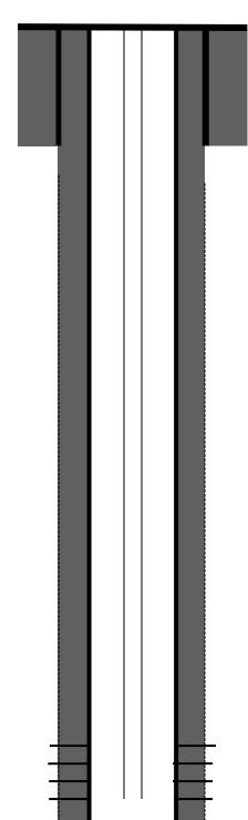
8-5/8" 23# casing @ 137'. Cemented with 100 sks. Hole size: 11"
