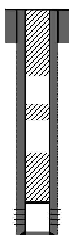
8-5/8" 23# casing @ 137'. Cemented with 100 sks. Hole size: 11"
