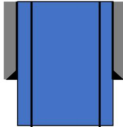
EOT @ 2290'. PUMPED 700SX CL C CMT TO SURFACE.
