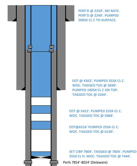
Borehole 11" Casing 8.625" SA 4210'
