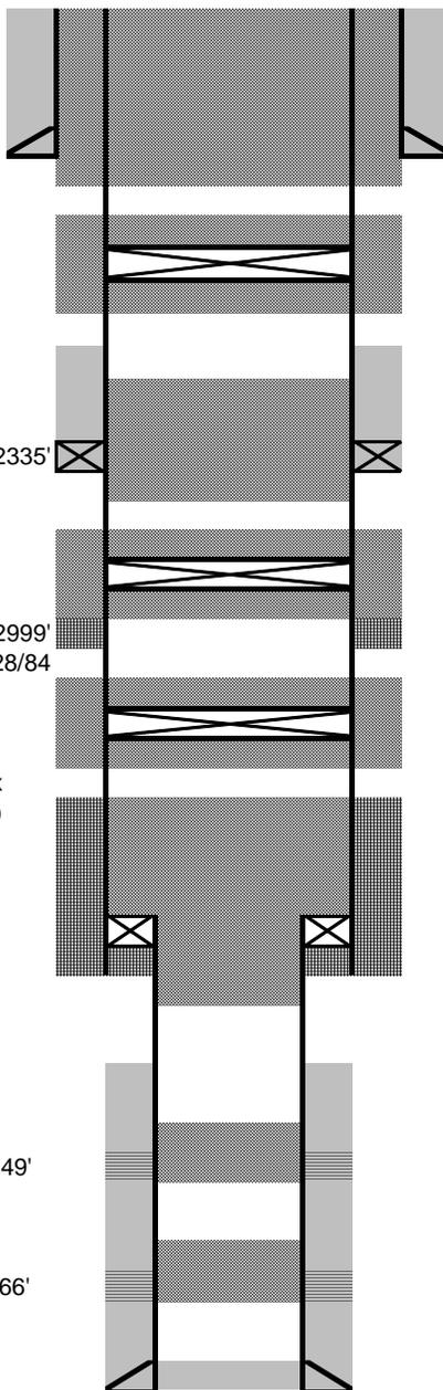
Plug 8: Surface casing shoe to surface: Perf holes at 319'. Tie onto 7" casing and mix and pump sufficient Class G cement to bring cement to surface, inside and outside 7" casing.
