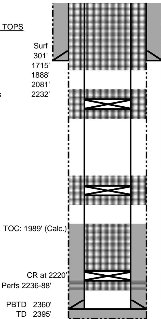
Plug 3: Surface shoe and surface plug: Perf holes at 265'. Tie onto 2-7/8" casing and mix and pump sufficient cement to bring TOC to surface, inside and outside.
