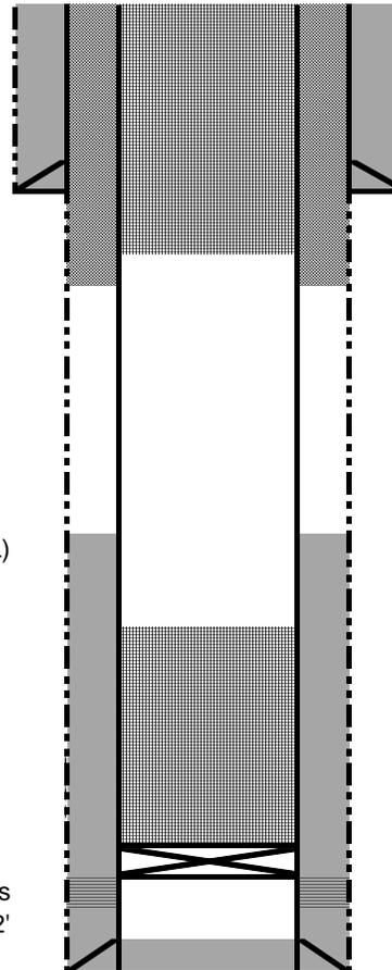
**Plug 2: Nacimiento, surface casing shoe, surface: Spot balanced plug from 513' to surface inside 4-1/2" casing. Top off cellar as necessary.**
