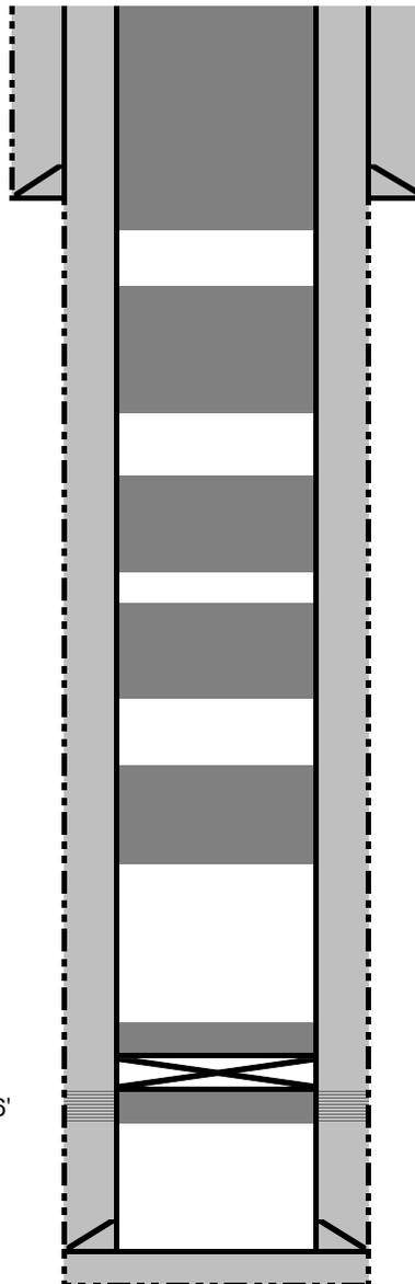
**Plug 6: Kirtland, Ojo Alamo, surface casing shoe and surface plug: Spot balanced plug from 1157' to surface.**
