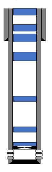
12-1/4" hole @ 1825' 9-5/8" csg @ 1825' w/ 1375sx-TOC-Surf-Circ
