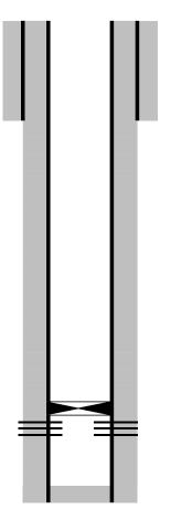
12-1/4" hole @ 715' 8-5/8"24# csg @ 705' w/ 400sx-TOC-Surf-Circ.
