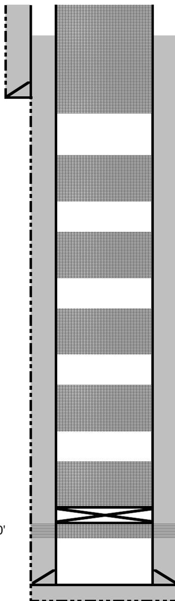
**Plug 6: Kirtland, Ojo Alamo, and surface plugs: Pending CBL results, it may be possible to top off cement at surface. If so, spot balanced plug from 307' surface. If not, shoot holes as indicated by CBL.**
