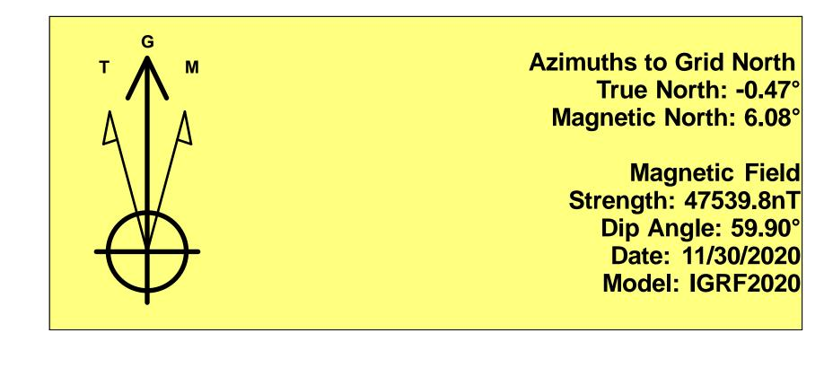
To convert a Magnetic Direction to a Grid Direction, Add 6.08° To convert a Magnetic Direction to a True Direction, Add 6.55° East To convert a True Direction to a Grid Direction, Subtract 0.47°
