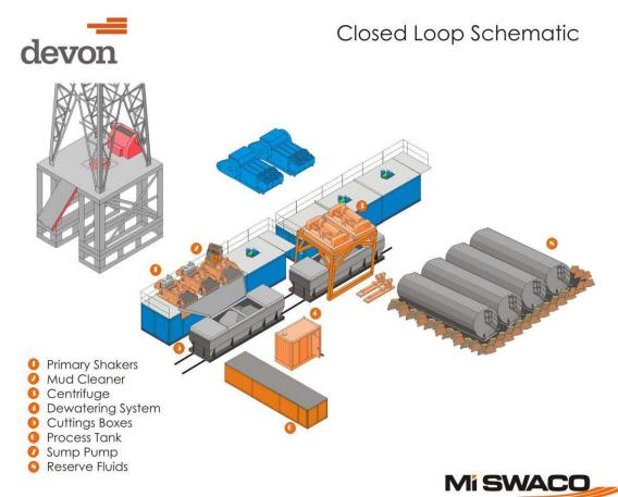
Centrifuges: The centrifuges can be one or two in number depending on the well geometry or depth of well. The centrifuges are sized to maintain low gravity solids at 5% or below. They may or may not need a dewatering system to enhance the removal rates. The centrifuges can make a cut point of 8-10 microns depending on bowl speed, feed rate, solids loading and other factors.
