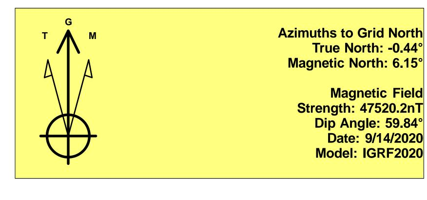
To convert a Magnetic Direction to a Grid Direction, Add 6.15° To convert a Magnetic Direction to a True Direction, Add 6.59° East To convert a True Direction to a Grid Direction, Subtract 0.44°
