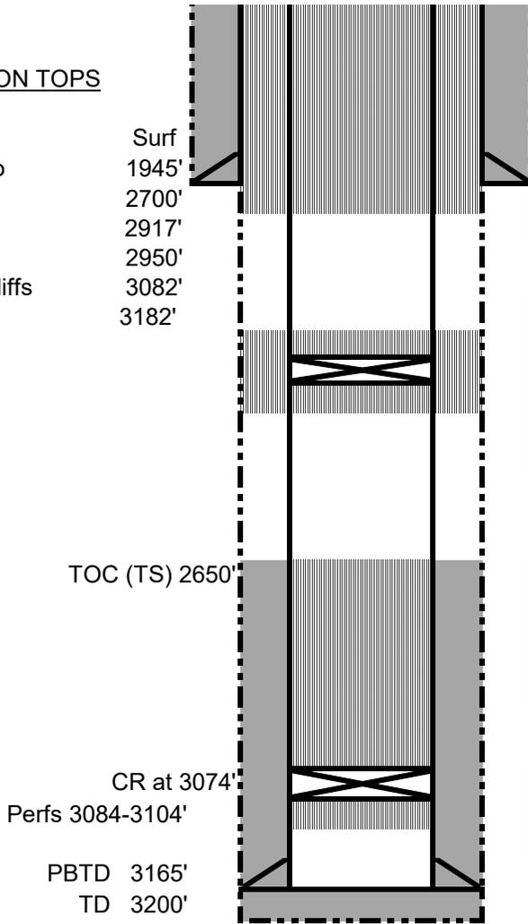
Plug 4: Surface shoe and surface plug: Perf holes at 188'. Tie onto 4-1/2" casing and mix and pump sufficient cement to bring TOC to surface, inside and outside.
