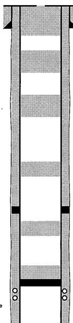
PBTD: 5950' TD: 5980' Hole Size: 12-1/4" 8-5/8", 24#, Casing set @ 363' Cement with 300 sx Class B, Circ 26 bbls to surface
