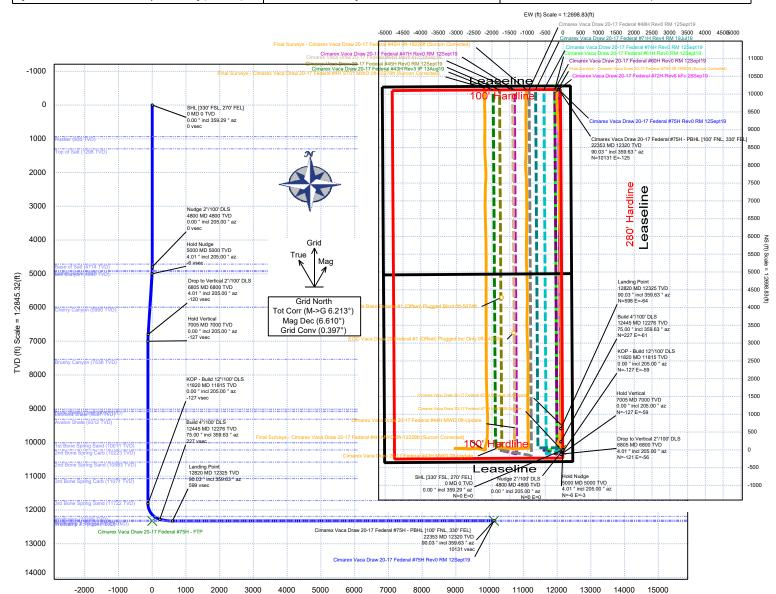
Vertical Section (ft) Azim = 359.63° Scale = 1:2845.32(ft) Origin = 0N/-S, 0E/-W
