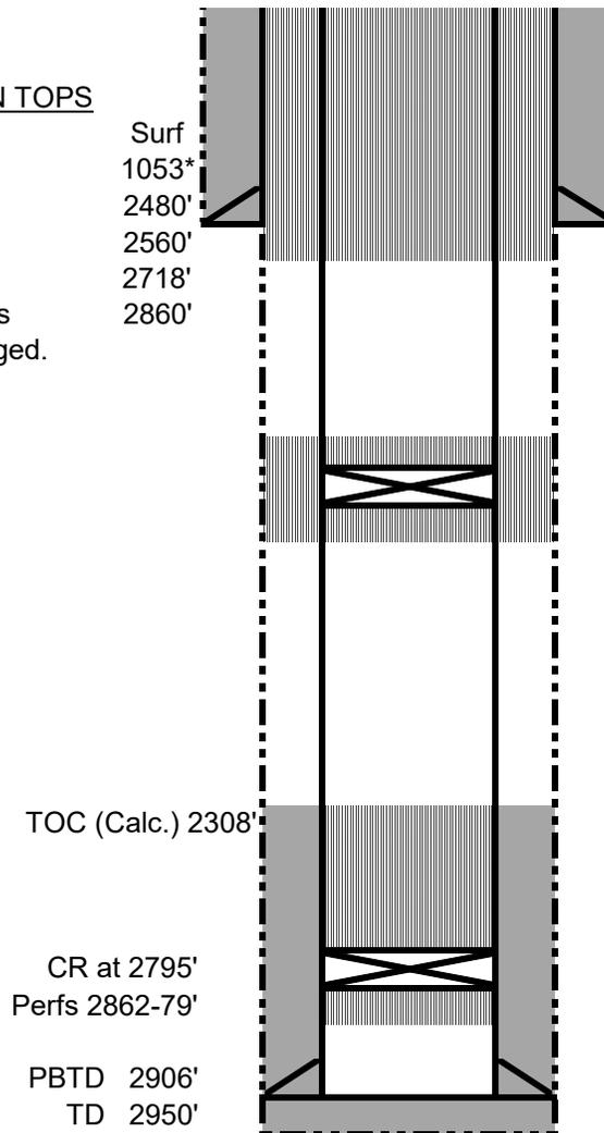
Plug 4: Surface shoe and surface plug: Perf holes at 152'. Tie onto 4-1/2" casing and mix and pump sufficient cement to bring TOC to surface, inside and outside.
