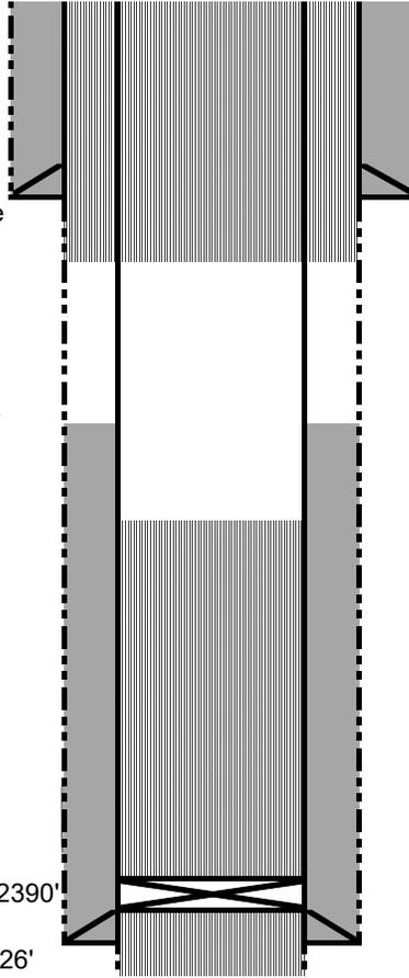
**Plug 3: Nacimiento, surface casing, and surface plug: Perf holes at 356'. Tie onto 5-1/2" casing and mix and pump sufficient volume to bring TOC to surface, inside and outside.**
