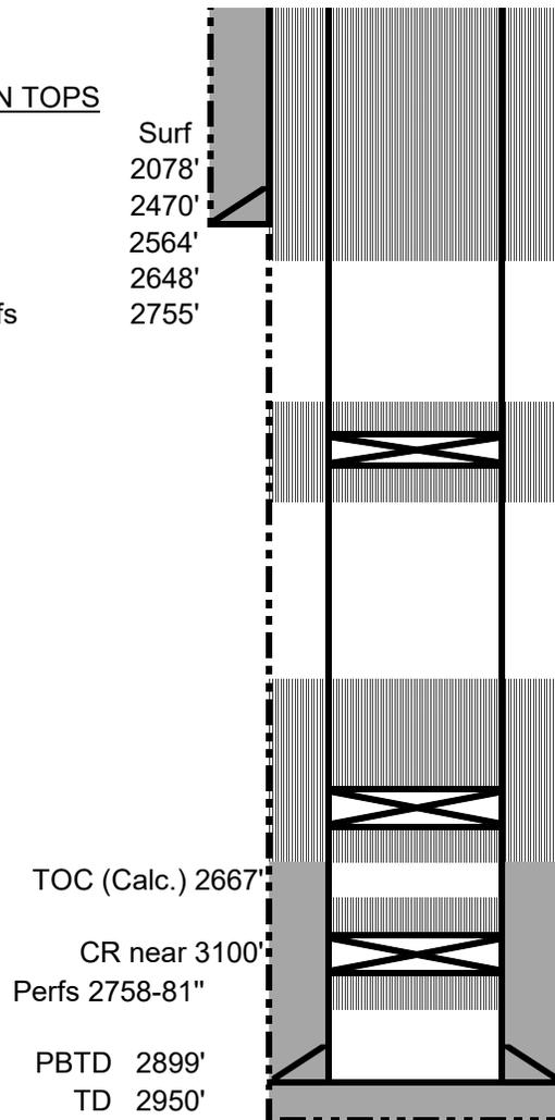
Plug 4: Surface shoe and surface plug: Perf holes at 186'. Tie onto 4-1/2" casing and mix and pump sufficient cement to bring TOC to surface, inside and outside.
