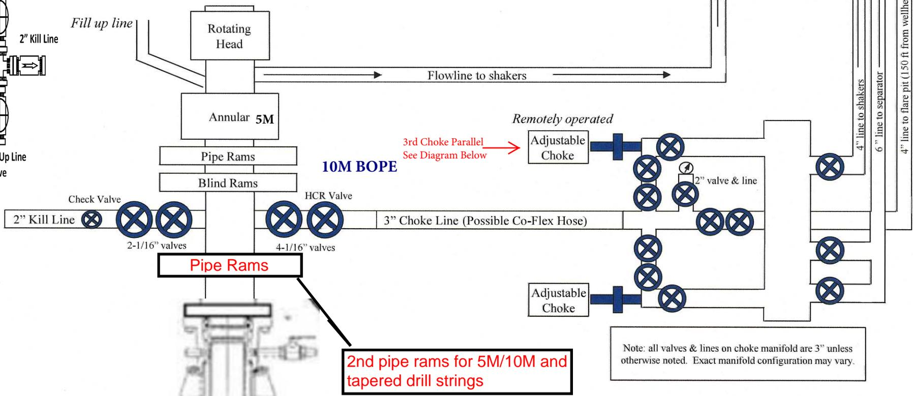
2nd pipe rams for 5M/10M and tapered drill strings
