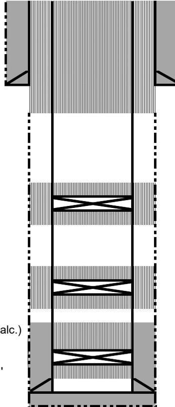
**Plug 5:** Surface casing shoe and surface: Perf holes at 154'. Tie onto 5-1/2" casing. Mix and pump sufficient cement to bring cement to surface inside and outside 5-1/2" casing.
