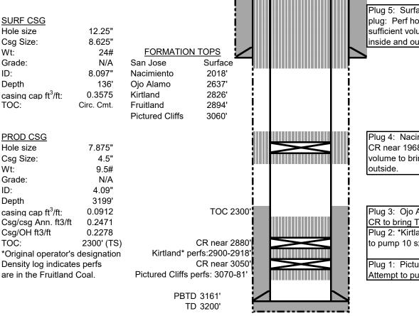
Plug 5: Surface casing shoe and surface plug: Perf holes at 186'. Mix and pump sufficient volume to bring cement to surface, inside and outside.
