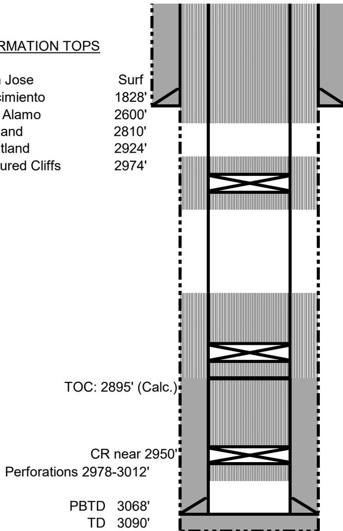
Plug 5: Surface shoe and surface plug: Perf holes at 150'. Tie onto 4-1/2" casing and mix and pump sufficient cement to bring TOC to surface, inside and outside.
