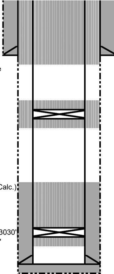
Plug 4: Surface casing shoe and surface plug: Perf holes at 172'. Mix and pump sufficient volume to bring cement to surface, inside and outside.
