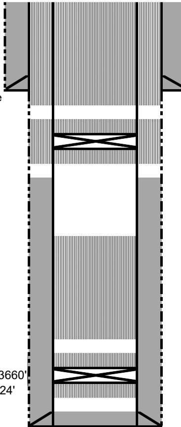
Plug 5: Surface casing shoe, surface: Perf holes at 303'. Mix and pump sufficient cement to bring TOC to surface, inside and outside.
