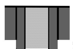
8-5/8" J-55 24# casing @ 279'. Cemented with 175 sks, 206.5 cf Class B w/ 3% CaCl2. Circulated 60 bbls to surface. Hole size: 12-1/4
