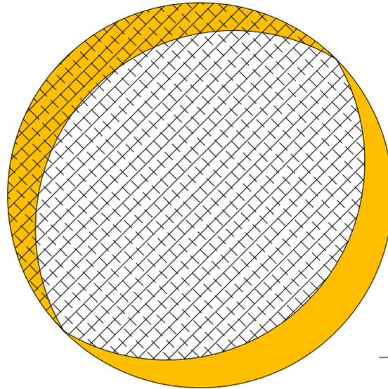
95 bbl steel tank: double wall / double bottom with leak detection port
