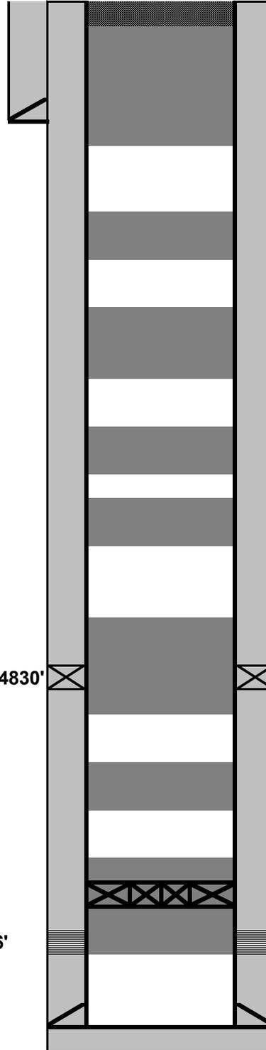
5-12-2022: Cut off WH, install P&A marker. TOC in 4 1/2" at 46', in annulus at surface. Mix top off of 24 sx for 4 1/2" and cellar.
