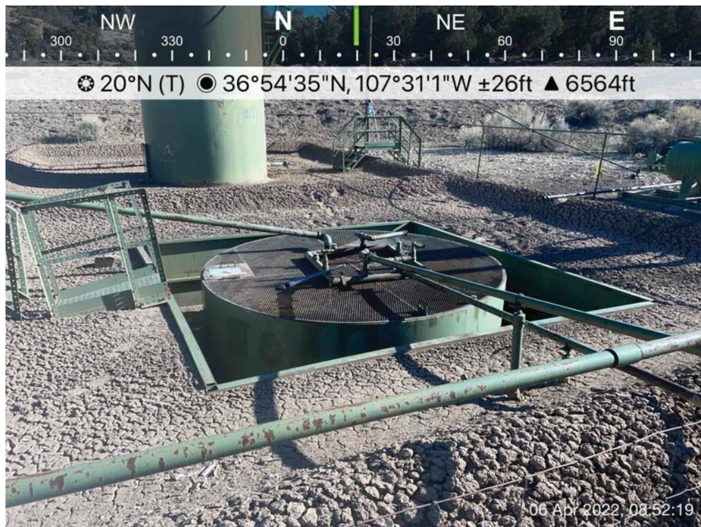
Photo 2: 80 bbls steel tank prior to removal, 4/6/2022.
