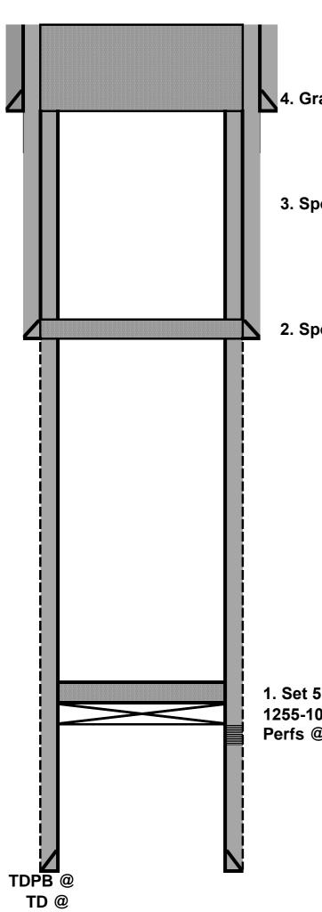
13 3/8 48# CSG @ 200 4. Gravity sqz'd 35 sx class C cmt @ 250' to surface.
