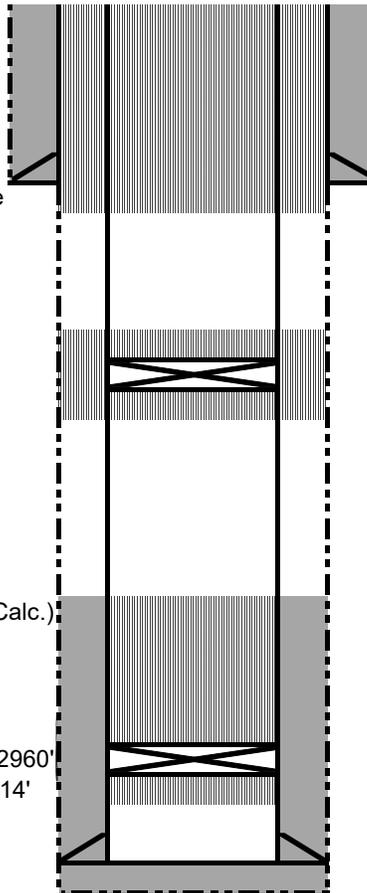
Plug 4: Surface casing shoe and surface plug: Perf holes at 150'. Mix and pump sufficient volume to bring cement to surface, inside and outside.
