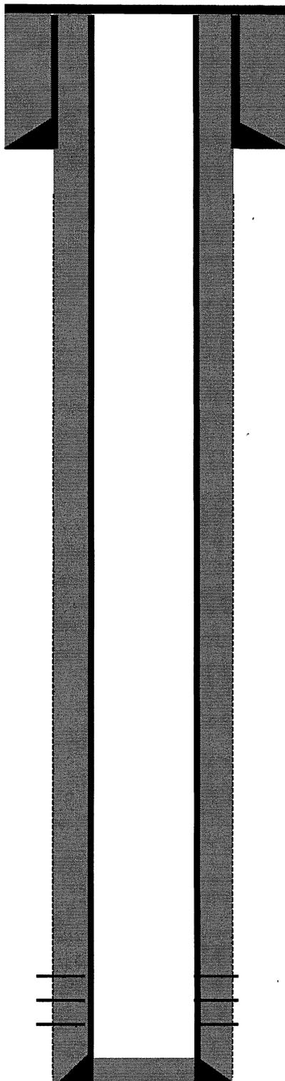
8-5/8" 24# J-55 casing @ 131'. Cemented with 95 sks Type 5 cement w/2% CaCl<sub>2</sub>. Circulated 3 bbls cement to surface. Hole size 12 1/4".
