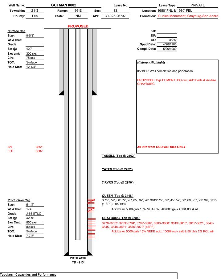
2-3/8" 4.7# J-55 Tubing (~119 jts 2-3/8" tubing, SN, 4' perf sub, MA w/ bull plug)
