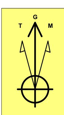
Azimuths to Grid North True North: -0.27° Magnetic North: 6.66°
