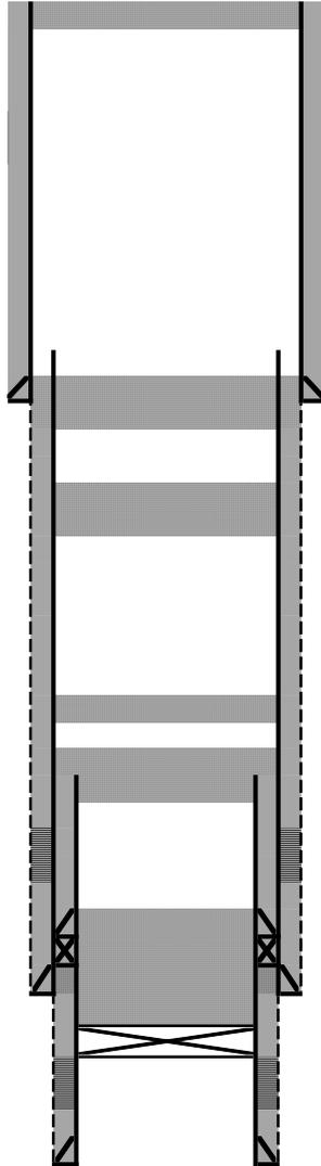
10. Cut off well head, verify cmt @ surface, weld on dry hole marker.
