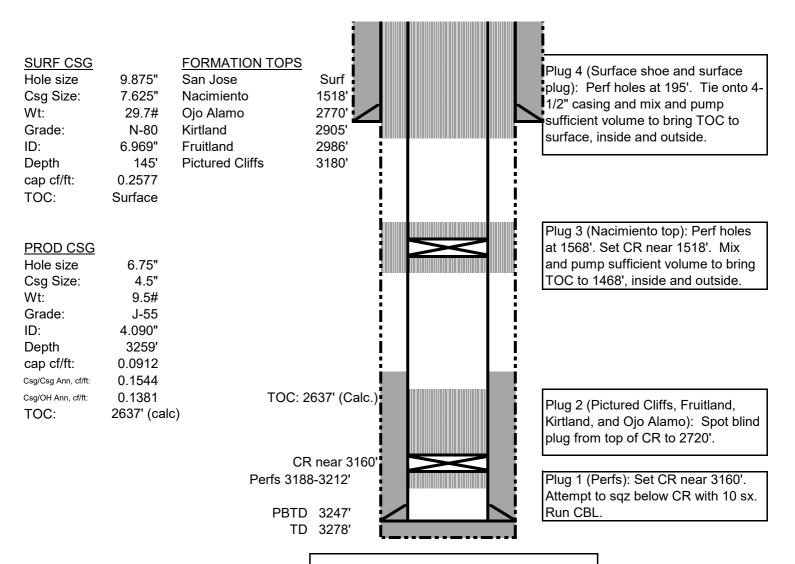
All plugs will include 50' excess cement inside pipe, and 100% excess outside.
