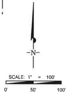
ALL BEARINGS, DISTANCES, AND COORDINATE VALUES CONTAINED HEREON ARE GRID BASED UPON THE NEW MEXICO COORDINATE SYSTEM OF 1983, EAST ZONE, U.S. SURVEY FEET. ELEVATIONS USED ARE NAVD88, OBTAINED THROUGH AN OPUS SOLUTION.
