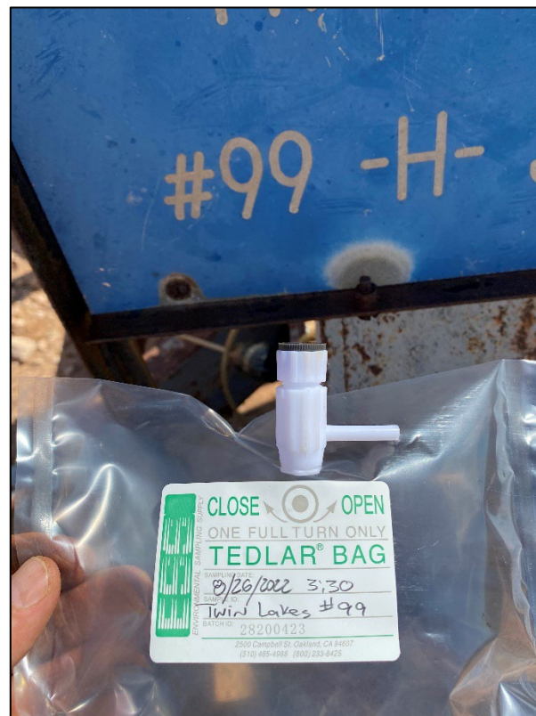
4) Twin Lakes SA #099 (30-005-61261) – Gas Sample Collection
